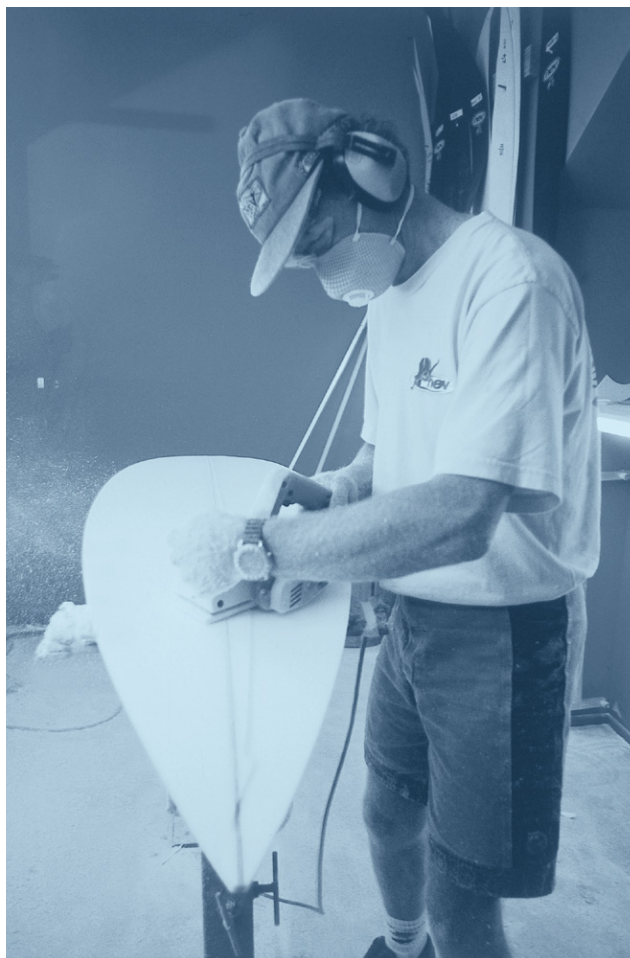
Figure 19.2 Surfboard blank being shaped
