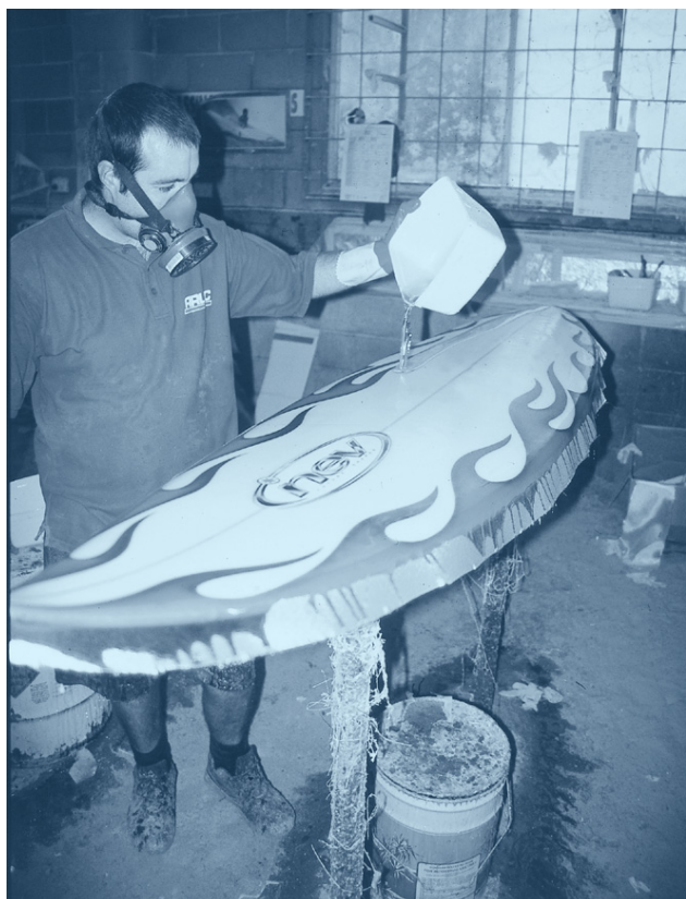
Figure 20.2 Applying filler resin to the fibreglass
