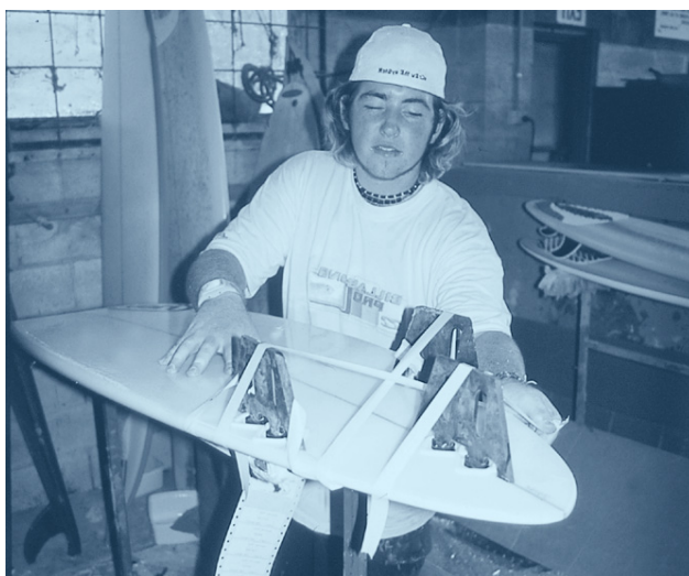
Figure 20.3 Adding the fin plugs. (Insert above: some tools used in the process)
